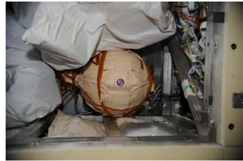
Fig.1. Liulin-5 onboard ISS. Upper-sketch of the detectors arrangement in the phantom, bottom- the spherical phantom, located in the MIM1 module. Inside the phantom (behind the label) is the detector block of Liulin-5.
